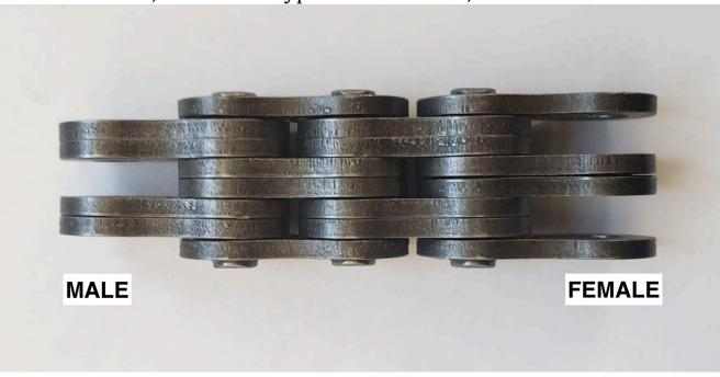
Depending on which pin is removed to separate the chain, the resulting end will be either Male or Female.
