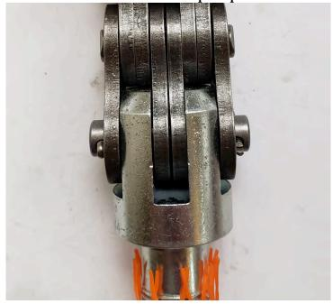
The final step in securing either the Connecting Link or Clevis Pin is to bend the split pin. The split pin does not take direct load and only needs to be bent enough to prevent it from falling out of the holes in
