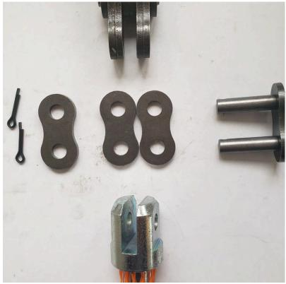
The independent plates need to be lined up in the same pattern as a Female chain end, in this case that means 1 plate on the outside, 2 plates on the inside and the plate with fixed pins on the far side.
